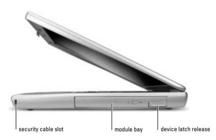
**SECURITY CABLE SLOT** — Lets you attach a commercially available antitheft device to the computer. For more information, see the instructions included with the device.
